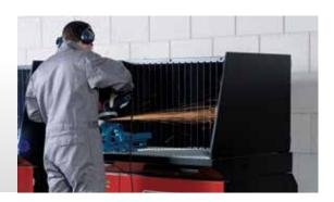
For optimum efficiency, it is necessary to adapt the speed of capture to the point of emission of fumes depending on the process used. Our team of fume control specialists will work on a solution that best meets your requirements.
